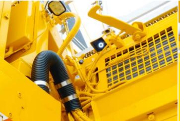
Camera monitoring of the slewing platform
