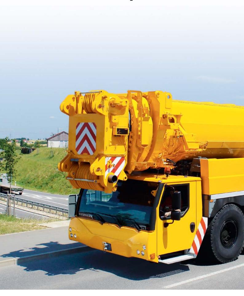
The LTM 1750-9.1 can carry the 52 m long telescopic boom, two folding outriggers and the main winch within the maximum axle load of 12 t. Considerable capacity increases are accomplished with the Y-telescopic boom suspension. Short set-up times, an extraordinary mobility as well as extensive comfort and safety appointments mark the mobile crane LTM 1750-9.1 from Liebherr.
