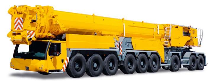
Total weight 108 t at 12 t axle load with front outriggers
