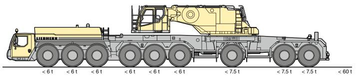
Without luffing cylinders and folding outriggers the total weight can be reduced to below 60 t.
