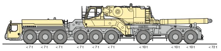
For axle loads below 10 t the telescopic boom is dismantled. One folding outrigger front left, the luffing cylinders and the hoist winch can be carried.
