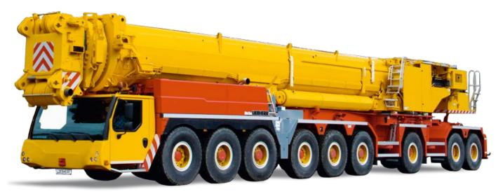
Total weight 99 t at 11 t axle load without outriggers
