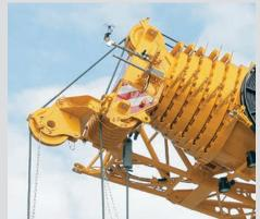
Hydraulic assistance for assembly of the swing-away jib with BTT
